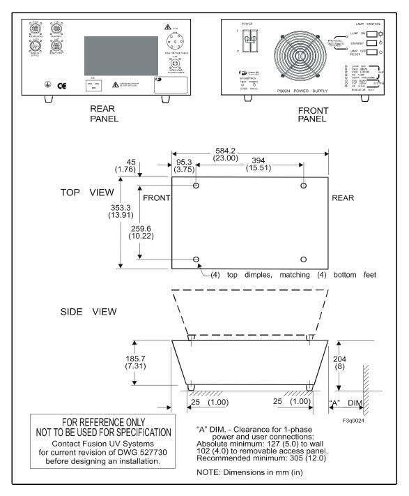
Figure 50. P300M/P300MQ Power Supply Dimensions and Clearances
